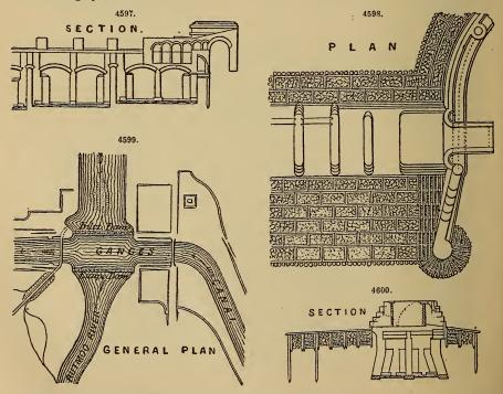
Regulators of smaller size will also be required at the head of each principal water-course, where it is taken off from the main line for irrigating purposes. A single opening will generally
